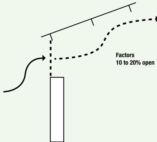
Perforated inlet material slows down air and gives a more even distribution. Gaps of 20-25mm between boards 50-200mm, to give an area 0.08m<sup>2</sup>/calf, are suitable for most houses. On exposed sites reducing the gap to 12mm and the space to 0.05m<sup>2</sup>/calf gives good results, especially if the house is not more than 12m wide.
