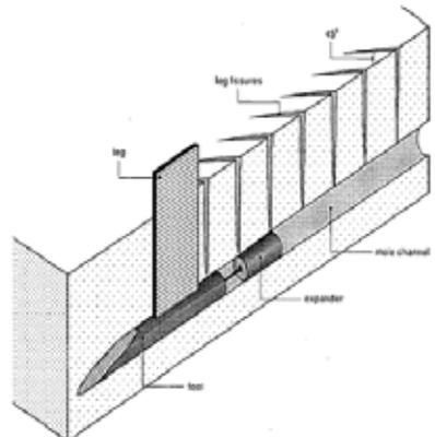
**Fig. 2b.** Cracking and channel formation
