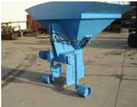
Fig. 3a. Gravel Mole plough showing hopper
