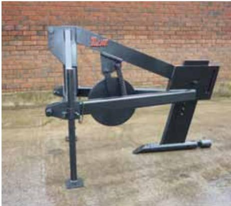
**Fig. 2a.** Mole plough showing cylindrical foot and expander.
