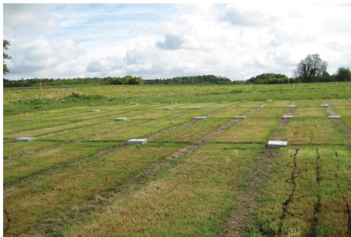
Measuring greenhouse gas emissions after application at the Teagasc Crops, Environment and Land Use Research Centre, Oak Park. The metal chambers are used for measuring gas emissions.
