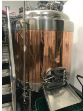
The brew process begins in the mill and then is transferred to the kettle for sterilisation.
