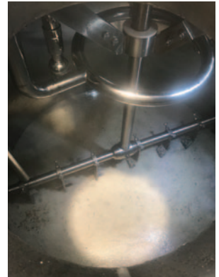
During this process enzymes convert starch in the grain into sugars.
