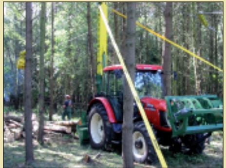
Specialised forwarding machines are the most common extraction system in Ireland. Similar to harvesters, forwarders can be fitted with tracks or chains and can remove on average 9-12 tonnes per journey.
