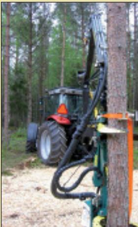
crane to the processing unit. Processors can debranch, cross-cut and stack timber assortments in the forest.
