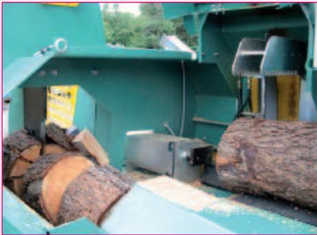
*A firewood processor will cut and split logs into suitable lengths.*
