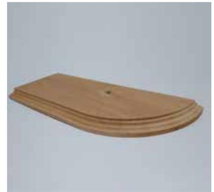
Figure 5 Test sample after CNC profile test.
