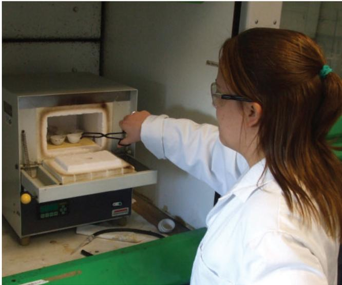
**Crucibles of test sample material being extracted from a muffle furnace at 550°C to determine their ash content.**
