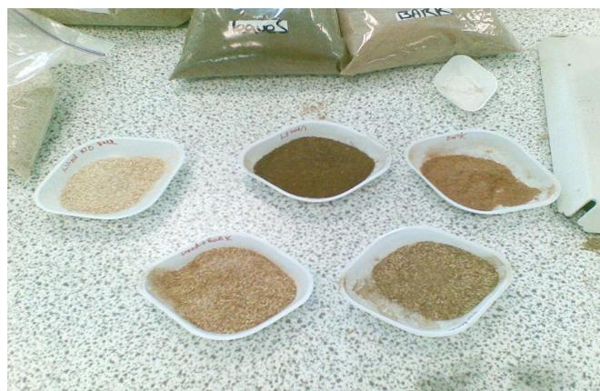
Figure 3. Ground wood, leaf, bark, roundwood and top samples for ash content and calorific value testing
