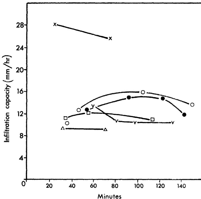
Fig. 4: Some typical infiltration curves after over-night wetting of the ground
