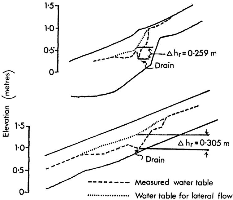
Fig. 7: Measured and estimated water-table elevations used in the calculation of radial resistance
