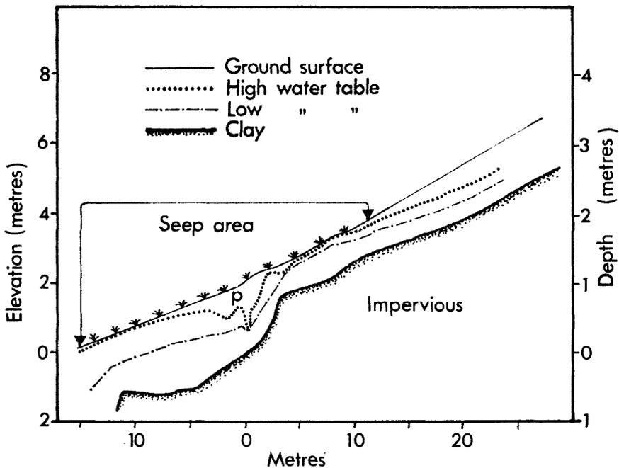
Fig. 5: Effect of the drain on water-tables where the drain was too low downhill to intercept the seepage
