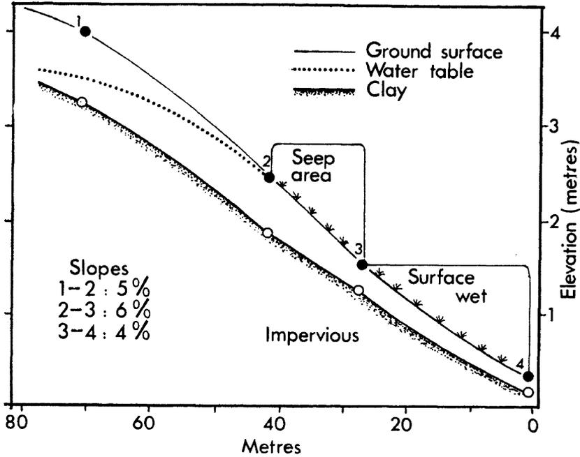
Fig. 1: A semi-section of a Killeshandra hillside showing the gradual constriction of the permeable layer and the occurrence of a seep zone
