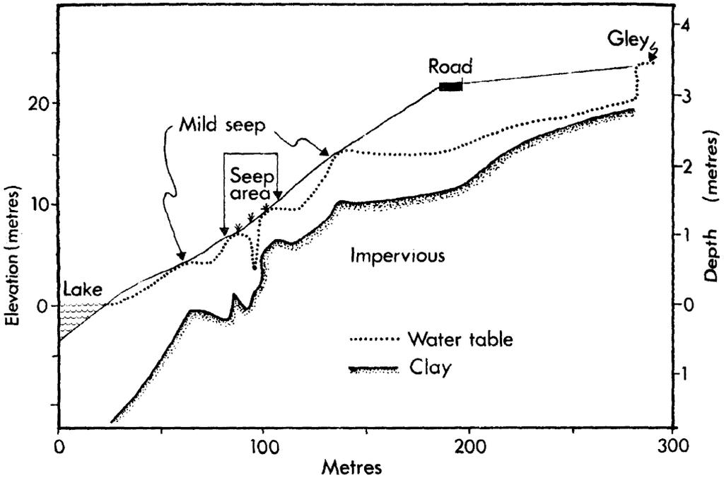
Fig. 2: A semi-section of a Killeshandra hillside showing the very uneven nature of the impervious clay layer and the occurrence of seepages
