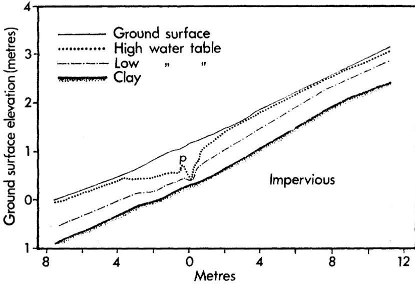
Fig. 6: Effect of the drain on water-tables where the drain seemed reasonably effective
