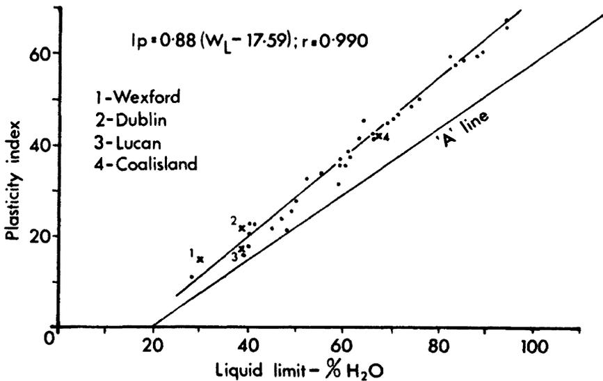
Fig. 1: Relationship of plasticity index to liquid limit of soils in North-central Ireland
