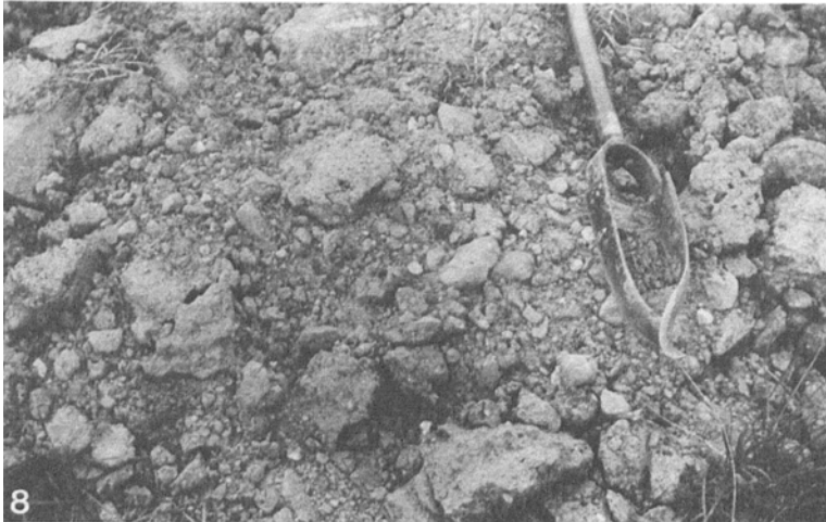
Figure 8. Permeability measurement can be difficult and tedious. This photo shows an 8-cm Dutch auger and an example of stony glacial till. The stones hamper augering and typically 3 out of 4 attempts to bore a hole to 1.2 m will fail on this type of soil.
