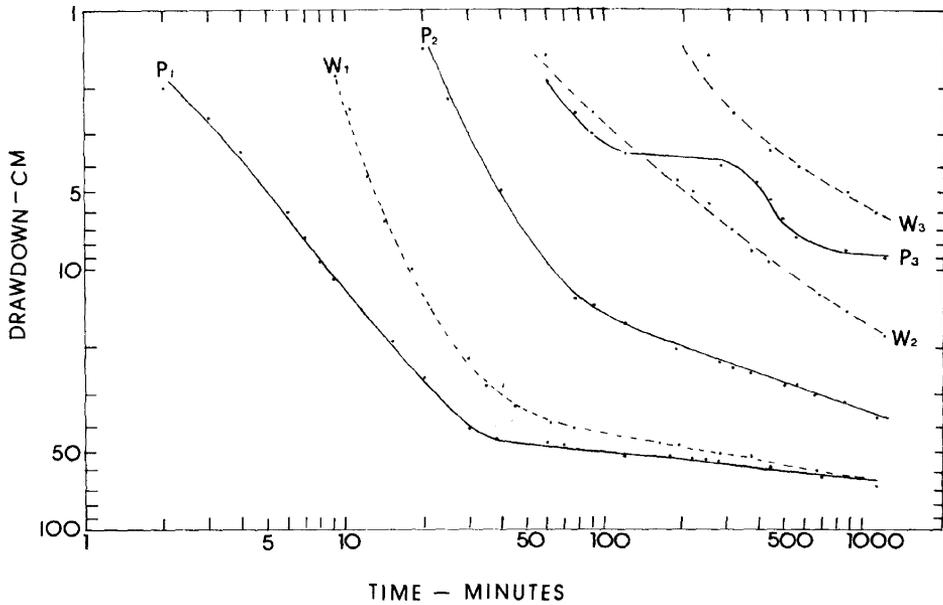
Fig. 4: Drawdown in the water-table and piezometer tubes with time; the subscripts 1, 2, and 3 refer to distances 7.5, 15 and 30 m from well
