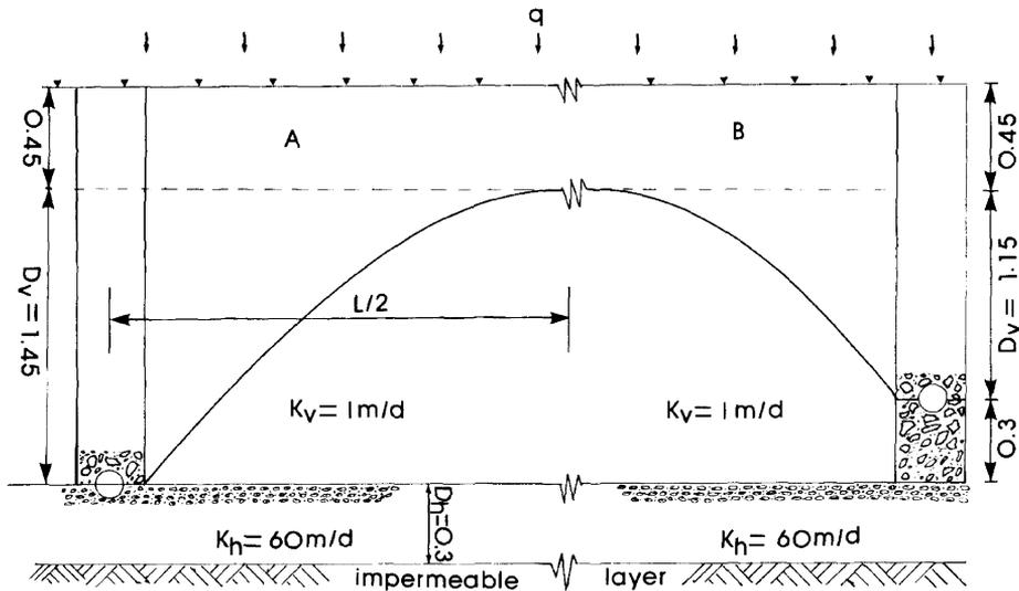
Fig. 5: Diagrammatic sketch showing geometry for the Ernst equation; Case A — drains at 1.9 m deep; Case B — drains at 1.6 m deep underlain by a connector gravel; all linear dimensions are in m
