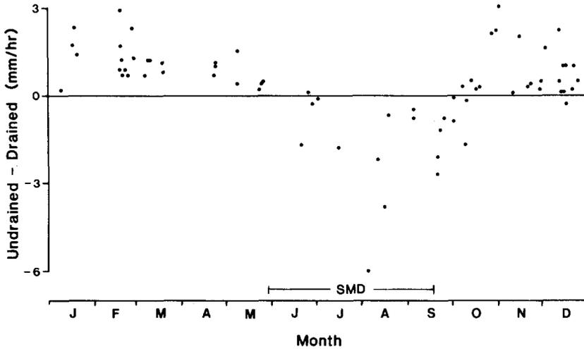
Fig. 5. Difference in peak hourly flows from the two plots at different times of the year. Data based on 70 storms, from June 1966 to November 1971. Points above the zero line indicate the undrained land yielded higher peaks in winter, whilst those falling below the line indicated higher peaks from the drained land in late summer. The average duration of soil moisture deficit is shown.
