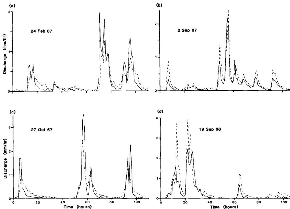
Fig. 4. Comparison of flows from the undrained (solid line) and drained (broken line) plots. In winter, (a) and (c), peak surface-layer flows from the undrained site were greater than maximum flows from the drained site. In late summer the drained-plot peaks were much larger, (b) and (d).
