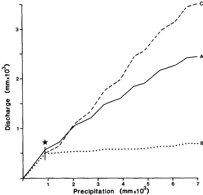
Fig. 1. Cumulative precipitation and outflow from the control plot (solid line, A) and experimental plot (broken lines) from November 1965 to October 1971 inclusive. The experimental plot was mowed in April 1966 (★) when the flows from the surface layer (B) and mole drains (C) were separately recorded.
