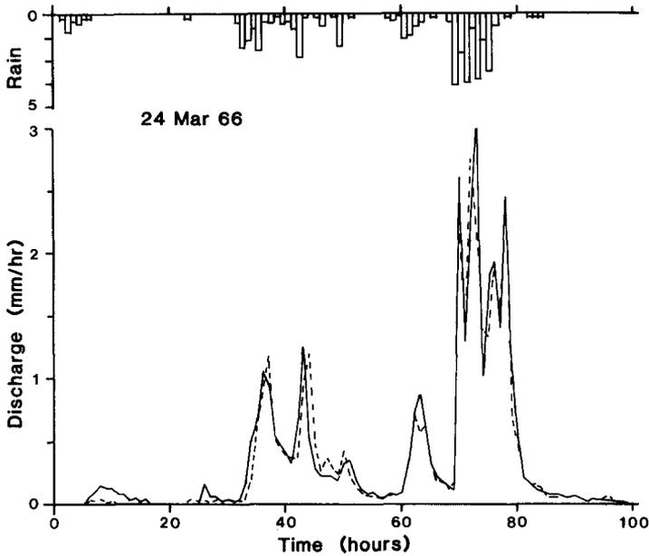
Fig. 3. Comparison of topsoil-layer storm flow from the control (solid line) and experimental (broken line) plots prior to drainage. Flows were derived as hourly totals, but for clarity are drawn as continuous curves.
