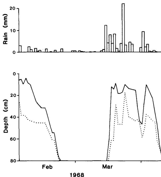
Fig. 2. Position of the water table on the undrained (solid line) and moled (dotted line) plots, based on daily-read tensiometers.
