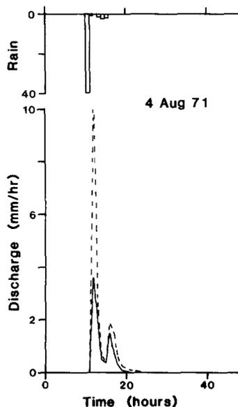
Fig. 6. Undrained (solid line) and drained (broken line) flows in response to a very intense summer thunderstorm.
