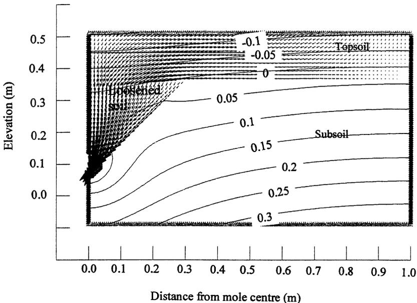
Fig. 6. Steady-state flow and pore-water pressure heads in soil with mole drains at 2.0 m spacing for a rainfall of 5 mm per day. Hydraulic conductivity values used were:  $K_{\text{topsoil}} = 3.0 \times 10^{-6}$  m/s,  $K_{\text{loosened soil}} = 0.5 \times 10^{-6}$  m/s and  $K_{\text{subsoil}} = 7.0 \times 10^{-10}$  m/s. The watertable is indicated by the zero pore-water pressure head contour.
