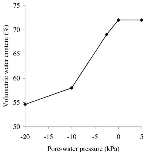
Fig. 3. Volumetric moisture content of topsoil against pore-water pressure (van Lanen and te Nuyl, 1997).
