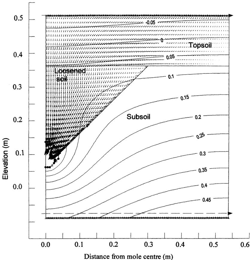
Fig. 5. Steady-state flow and pore-water pressure heads in soil with mole drains at 1.075 m spacing for a rainfall of 12 mm per day. Hydraulic conductivity values used were:  $K_{\text{topsoil}} = 3.0 \times 10^{-6}$  m/s,  $K_{\text{loosened soil}} = 0.5 \times 10^{-6}$  m/s and  $K_{\text{subsoil}} = 7.0 \times 10^{-10}$  m/s. The watertable is indicated by the zero pore-water pressure head contour.
