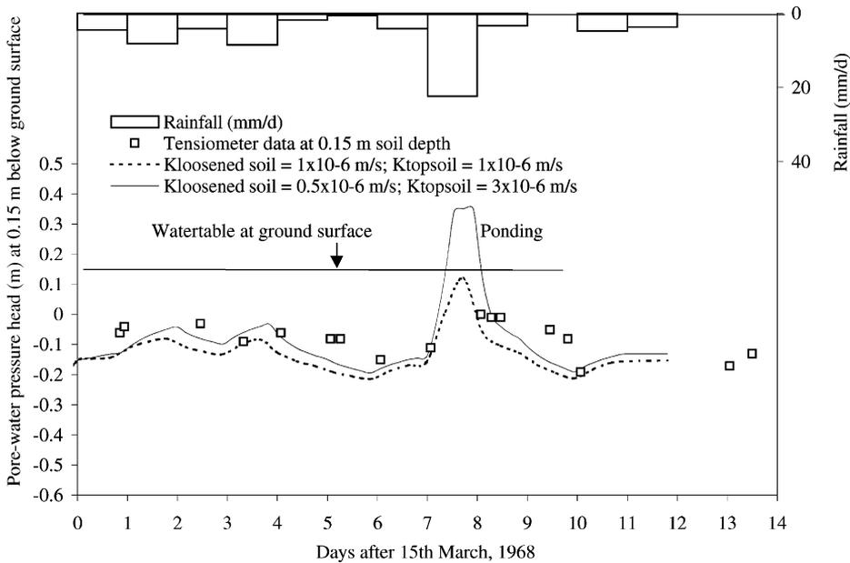
Fig. 4. Comparison of pore-water pressure heads (m) at 0.15 m below ground surface from SEEP/W analyses and tensiometer field measurements midway between mole drains at 1.07 m centres using rainfalls over 12 days in March 1968.
