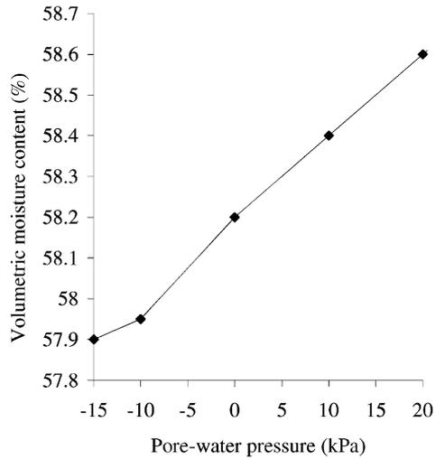
Fig. 2. Volumetric moisture content of clay subsoil against pore-water pressure (Mulqueen, 1990; GEO-SLOPE, 2001).
