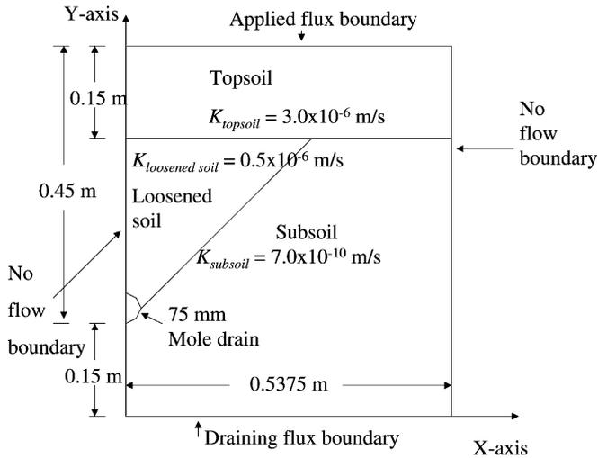
Fig. 1. Geometry and boundary conditions of a vertical semi-section of soil used in the finite element model with mole drains spaced at 1.075 m centres.
