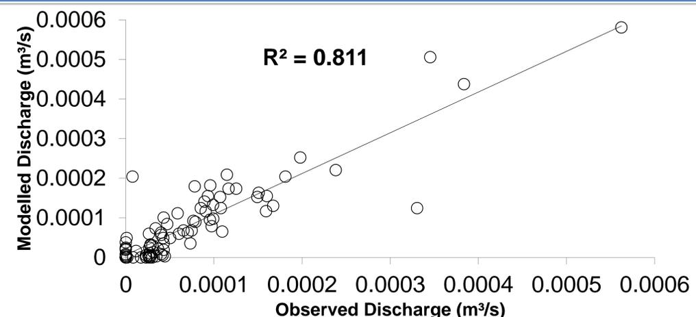
**Figure 1. Modeled vs. observed daily tile drain discharge (m<sup>3</sup>/s) from System 1 during the validation event (Event B). Index of Agreement = 0.94**
