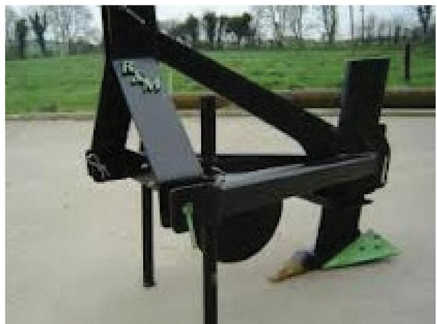
**Figure 5: Single leg winged sub-soiler.**
