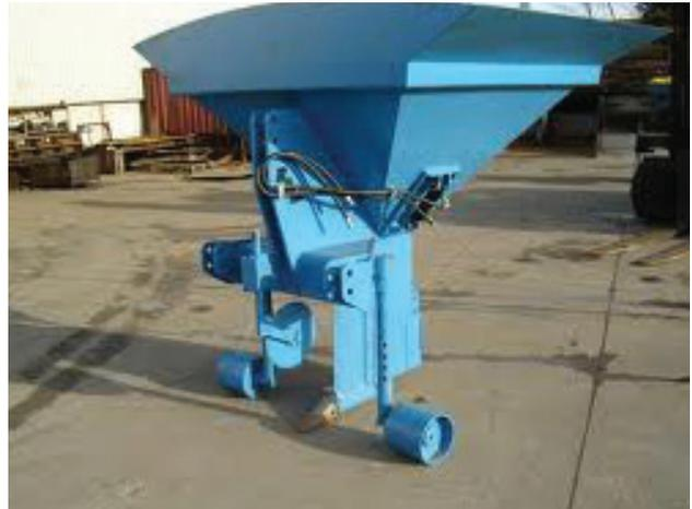
**Figure 4: Gravel mole plough showing hopper.**
