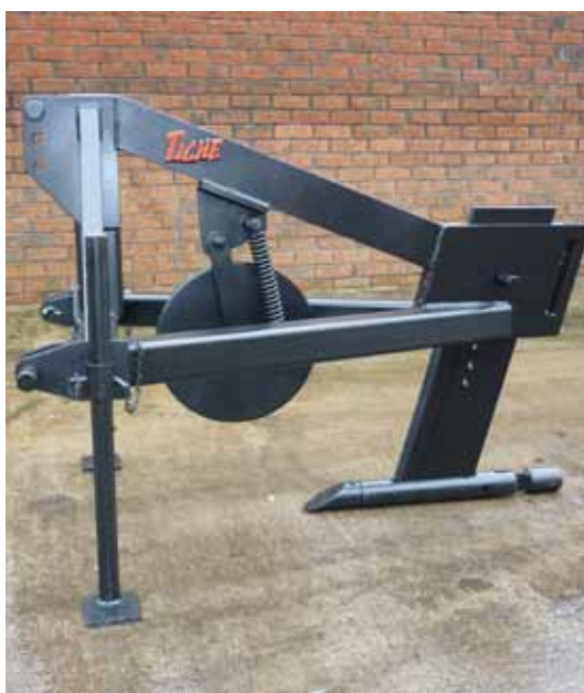
Figure 3. Mole plough showing cylindrical foot and expander
