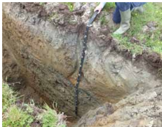
Figure 1. Test pit excavation
