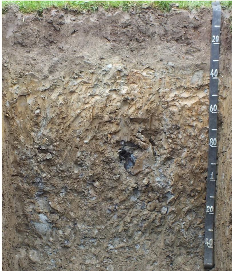
Figure 16. Paddock 17, 0700 Typical Surface-water Gley, series Kilrush. Fine Loamy drift with siliceous stones.
