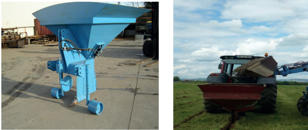
Fig. 3a. Gravel Mole plough showing hopper, 3b. Operation and filling of gravel mole plough
