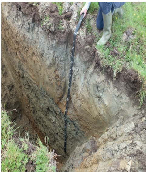
Fig. 1a .Test pit excavation
