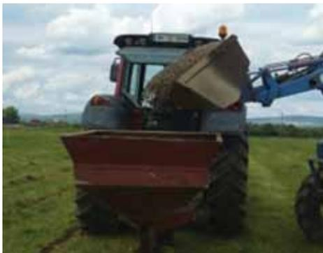
Fig. 3b. Operation and filling of gravel mole plough
