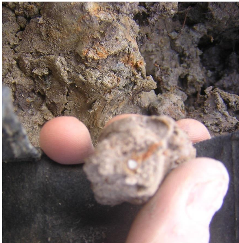
Plate 16. Cross section through coarse roots of the rushes found in this field. The plant can bring oxygen to anoxic layers. As a consequence of the oxygen at depth, iron has precipitated out in the area surrounding the root – orange/red colour.
