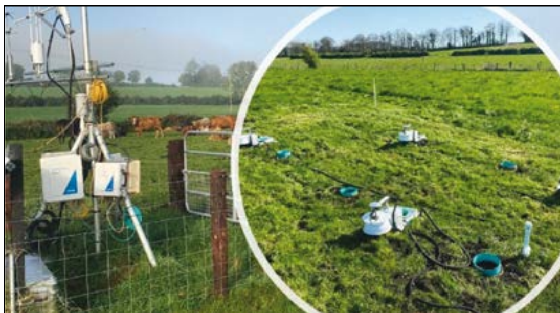
Figure 2: An eddy covariance tower and auto-chamber experiment investigating the impacts of water table management (WTM) on carbon (C) and greenhouse gas (GHG) dynamics on an agricultural peat-based grassland. Images provide by Ian Clancy.
