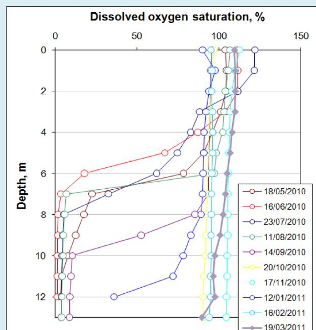
Fig. 4 Dissolved Oxygen Profile in Sreenty Lough
