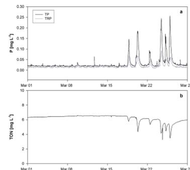
Fig. 4. Dynamic patterns of a) P fractions and b) TON concentrations in streamflow captured by bankside analysis
