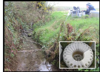
Fig. 3. Traditional autosamplers are usefully deployed in difficult to access streams
