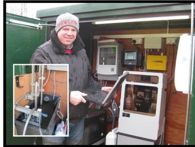
Fig. 2. Bankside analysis provides sub-hourly measures of stream TP, TRP, TON, conductivity, temperature and turbidity
