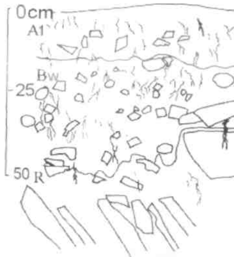
Figure 4.6: Profile drawing of Ballylanders Series (Brown Earth) developed over shale bedrock (see Fig. 4.2 for explanation of symbols).
