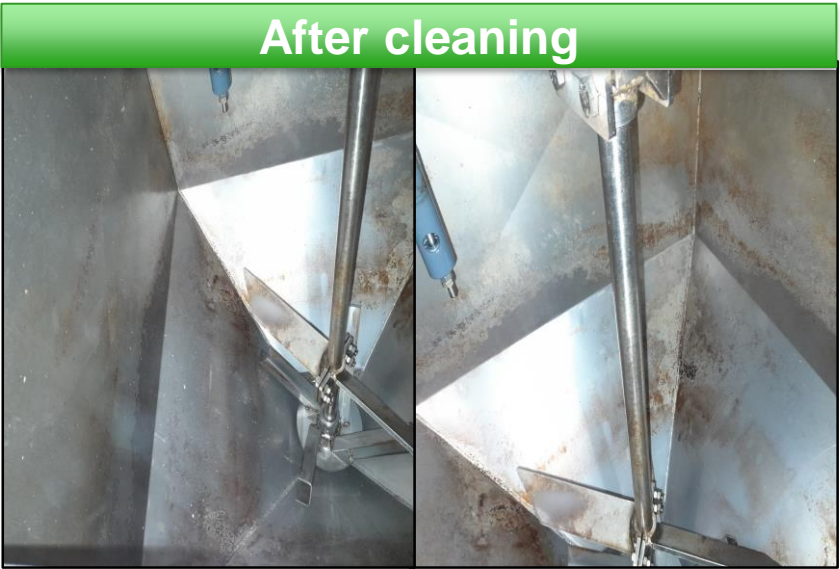
Mixing tank scrubbed and power washed
