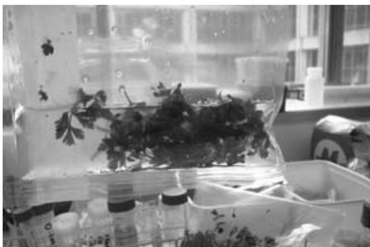
**Figure 7: Parsley following Pulsification for 1 minute. As can be seen there is very little breakdown of this leaf crop caused by the action of the Pulsifier.**
