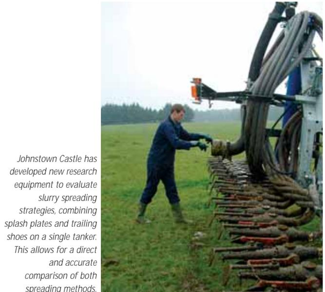
*Johnstown Castle has developed new research equipment to evaluate slurry spreading strategies, combining splash plates and trailing shoes on a single tanker. This allows for a direct and accurate comparison of both spreading methods.*
