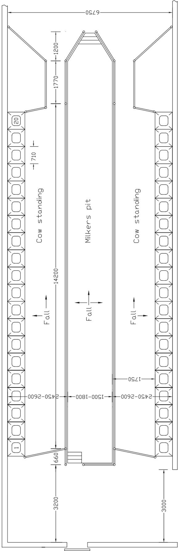
Drawing 4. 20 unit side-by-side parlour with sequential bailing and auto identification
