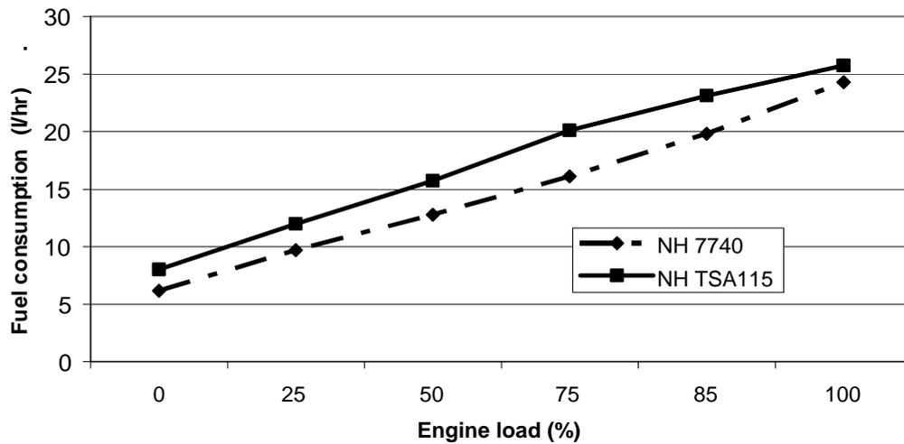
**Fig 5:** Tractor fuel consumption for newer and older tractor models at 80kW power output
