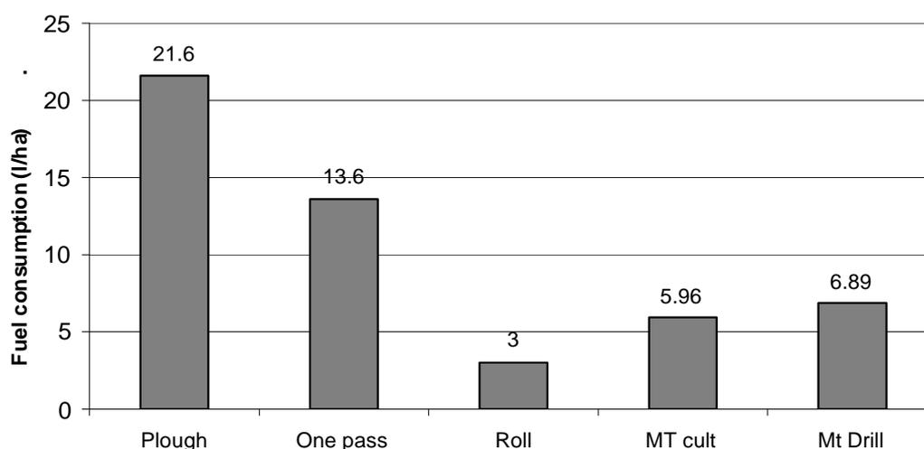
**Fig 2:** Estimated fuel consumption for different cultivation operations.
