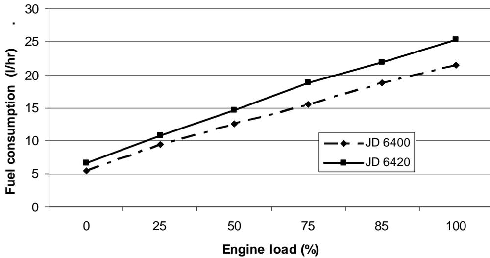
**Fig 4:** Tractor fuel consumption for newer and older tractor models at 80kW power output
