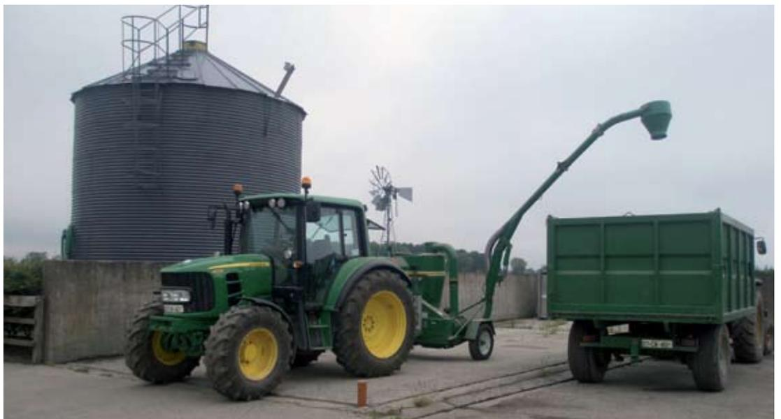
**Image 23:** Grain sucker/blower. This is a very versatile machine for handling grain. It can load and unload grain to and from trailers, trucks, bins and flat stores. The blower work rate is about 35 tonnes per hour. There is also a portable suction head to clean up the last of the grain from the yard or store.
