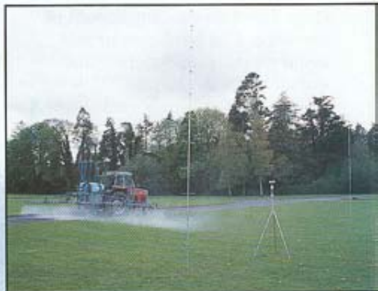
Spray drift measurement at Teagasc, Oak Park.
