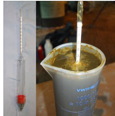
Figure 2. Slurry hydrometer with graduated scale used to estimate the slurry dry matter content in a well mixed slurry sample.
