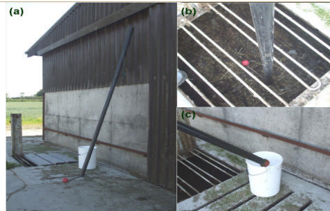
Figure 1. 'Tube sampler' consisting of a 6 cm diameter plastic pipe with a rubber ball stopper attached to a rope that runs through the centre of the pipe (a). The tube is inserted to the full depth of the unagitated slurry tank (b) and the ball stopper is applied to the end of the pipe by pulling the rope. The full column of slurry is then extracted from the tank by securing the rope to hold the ball stopper in place. The extracted column of slurry can be collected in a vessel by releasing the ball stopper (c).
