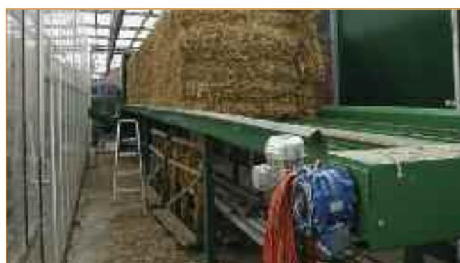
Straw bales being fed into shredder and combustion chamber.
