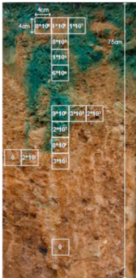
Figure 1 Soil flow paths stained blue with E. Coli concentrations superimposed in white.
