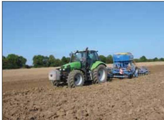
Proper matching of tractors and implements will result in more efficient engine loading and lower fuel use
