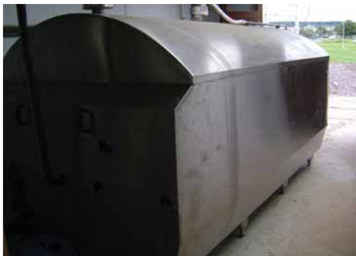
Bulk tank requires heated water for cleaning
