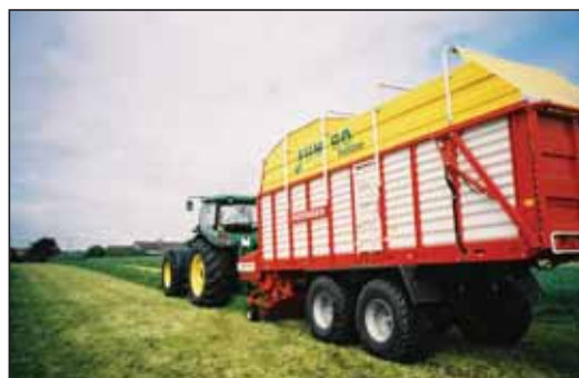
The pick-up wagon system requires less power and uses less fuel than precision chop systems.
