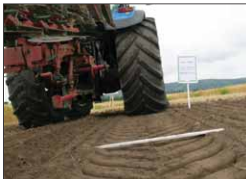
Wider tyres sink less and have a lower rolling distance in the field
