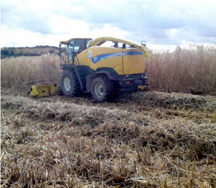
Self propelled harvester with a Kemper header which is cutting and crimping miscanthus into a sward prior to baling.
