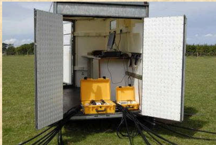
Three mobile laboratories – each containing an automated soil CO 2 flux system with 12 chambers
