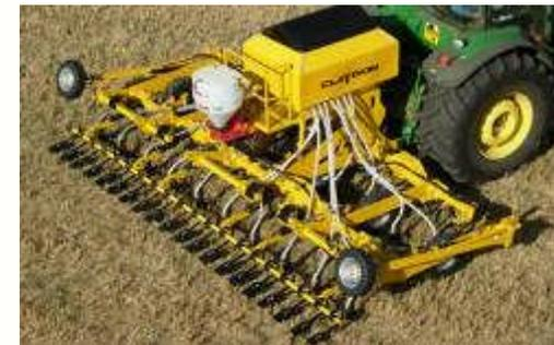
Example of a direct seed drill. This one-pass crop establishment drilling method allows a farmer to drill cereals (wheat, barley), rape seed (rape, linseed) and pulses (maize, peas, beans) directly into stubble, minimum-tilled or fully cultivated land.
