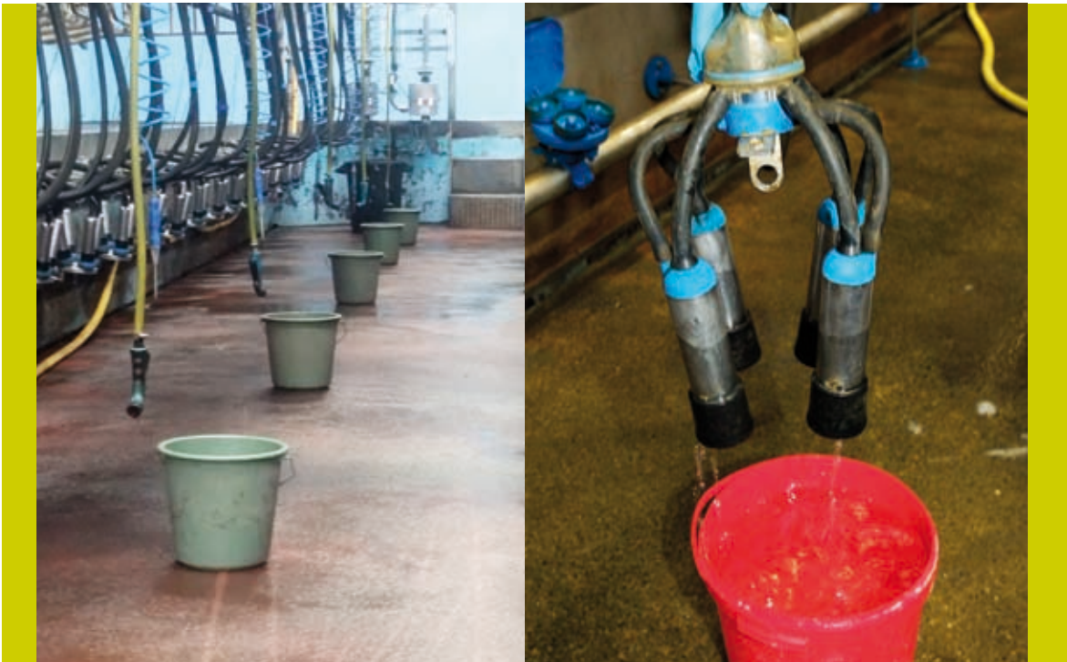
Typical cluster dipping layout in parlour pit.
