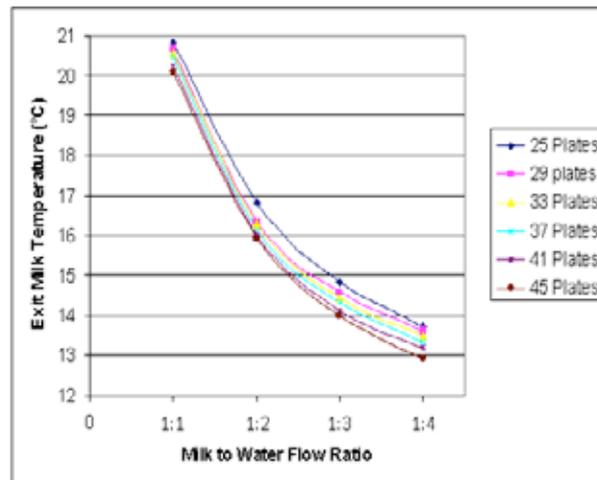
**Figure 2:** Milk exit temperature for varying ratios and PHE capacities.
