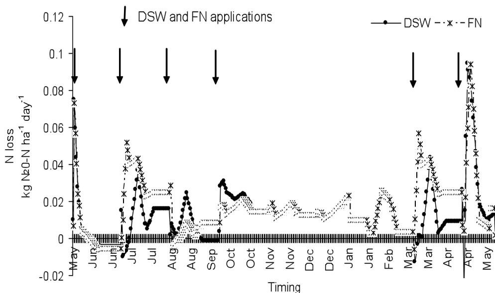
Figure 2: Seasonal patterns of  $N_2O$  fluxes (arrow indicates DSW application in tandem with FN)
