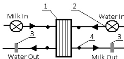
Figure 1: PHE test rig: 1-PHE, 2-Variable Speed Pump, 3- Ultra Sonic Flow Meter, 4- Type K Thermocouple
