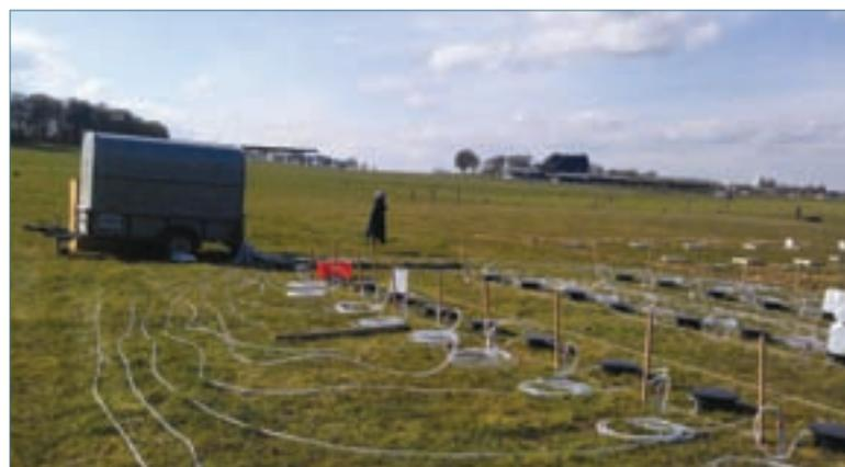
Figure 2: Dynamic chambers deployed for ammonia measurements.
