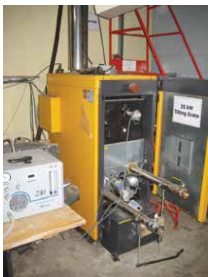
Air Staging Experimental Set-up
