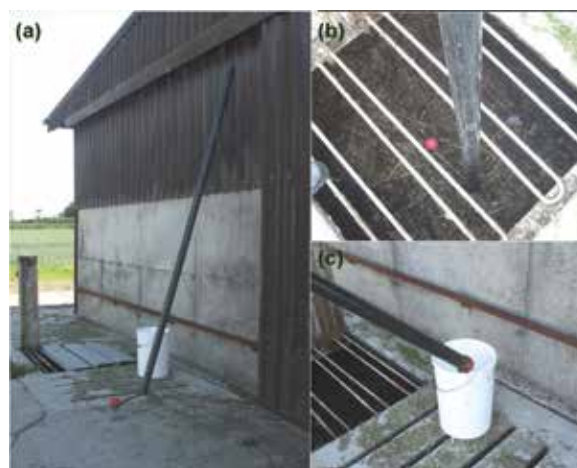
Figure 1. 'Tube sampler' consisting of a 6 cm diameter plastic pipe with a rubber ball stopper attached to a rope that runs through the centre of the pipe (a). The tube is inserted to the full depth of the unagitated slurry tank (b) and the ball stopper is applied to the end of the pipe by pulling the rope. The full column of slurry is then extracted from the tank by securing the rope to hold the ball stopper in place. The extracted column of slurry can be collected in a vessel by releasing the ball stopper (c).
