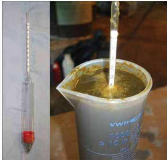
Figure 2. Slurry hydrometer with graduated scale used to estimate the slurry dry matter content in a well mixed slurry sample.
