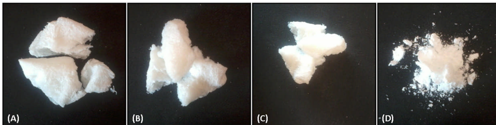
Gelatin generated with the NaCl method: (A) Salmon Bones, (B) Salmon Skin, (C) Salmon Heads and (D) Salmon Offal
