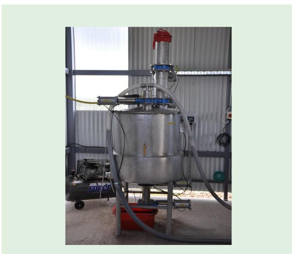
Figure 1. Pilot-Scale Anaerobic Digester located at Teagasc, Moorepark
