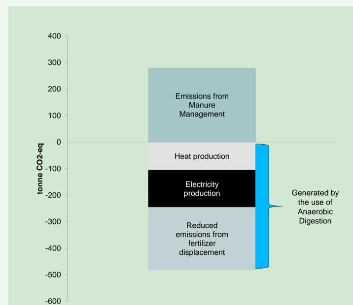
Figure 2. GHG emissions from a typical Irish pig farm and GHG mitigation potential of anaerobic digestion
