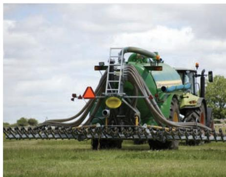
*The Low Emission Slurry Spreading Equipment Scheme covers slurry tankers using a trailing shoe spreader.*
