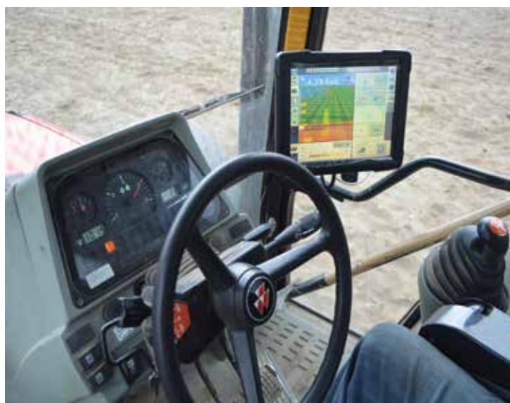
The display unit in the cab shows the operator where the plot lines are but steering and seeder control are completely automatic, eliminating the need for time-consuming marking out and accurate operator steering.
