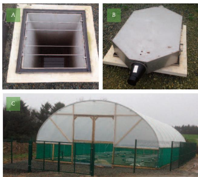
FIGURE 2: New slurry storage facility at Teagasc Johnstown Castle showing: (a) one of twelve 1m<sup>3</sup> concrete storage tanks; (b) dynamic chamber used to measure ammonia and greenhouse gas emissions; and, (c) overview of the facility.
