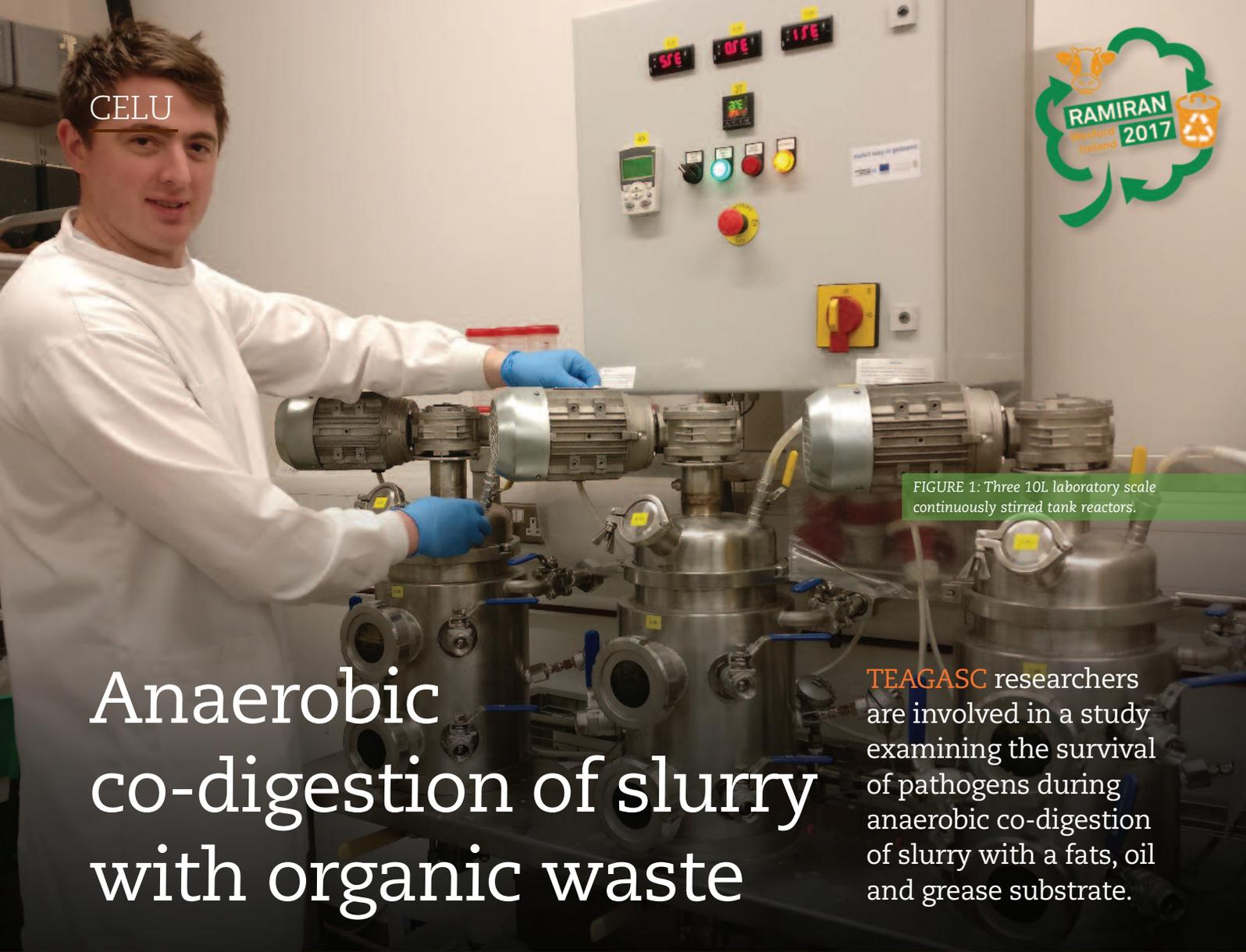
FIGURE 1: Three 10L laboratory scale continuously stirred tank reactors.
